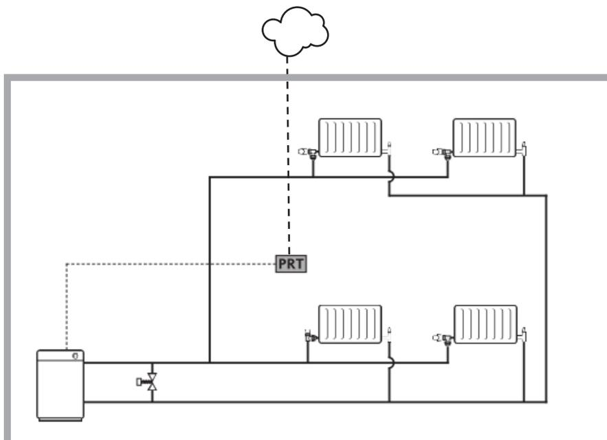
Programmable room thermostat and thermostatic radiator valves
