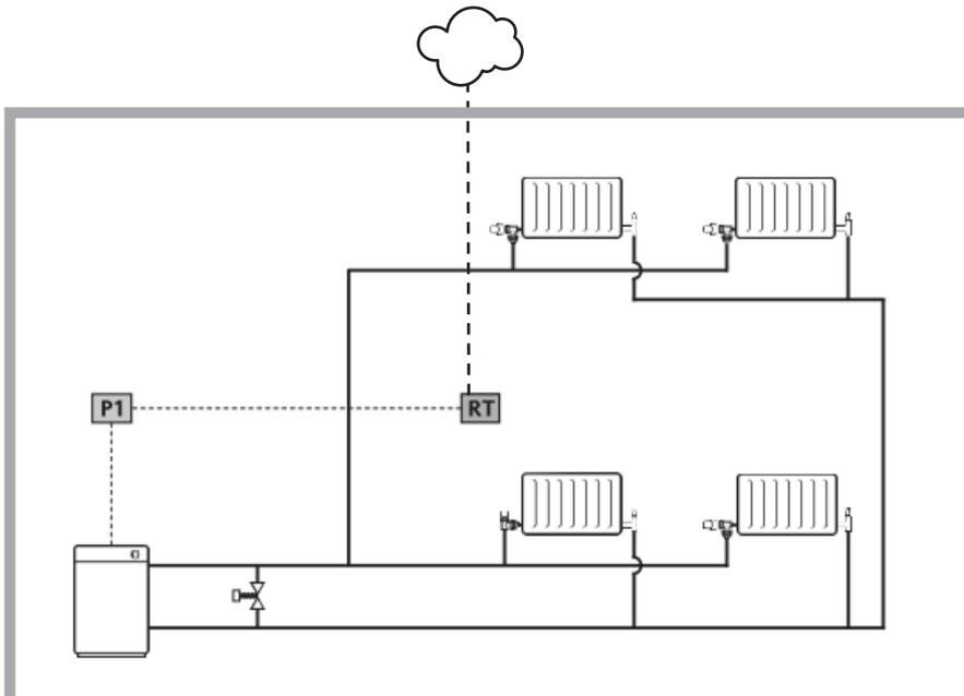
Programmer, room thermostat and thermostatic radiator valves
