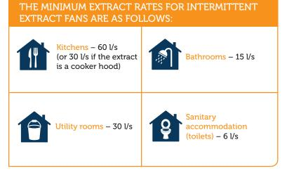
**NOTE:** The stated extract rate of a fan may be lower when installed due to resistance from ductwork, grilles etc. It is the installer's responsibility to ensure that the fan can deliver the required extract rate for the room once the installation is complete.
