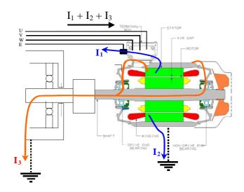
Figure 12 - Earth paths for high-frequency current
