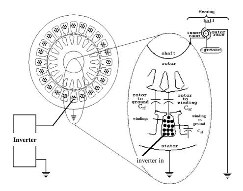
Figure 9 - Capacitances of motor winding
