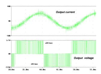
Figure 6 - Typical PWM voltage and current motor waveforms
