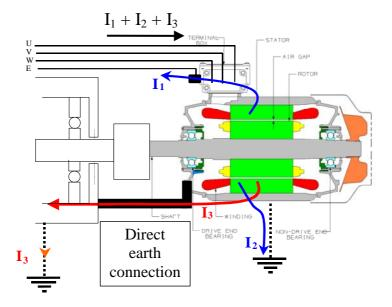
Figure 15 - Addition of direct earth connection between motor and driven machine, to prevent shaft grounding current
