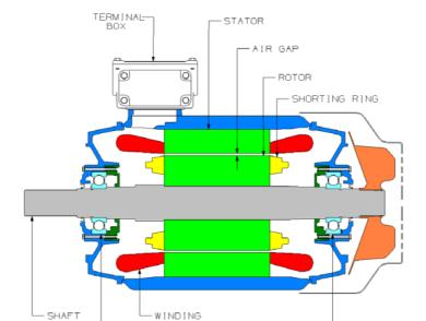
Figure 1 shows a longitudinal view of an induction motor with its constituent parts.
