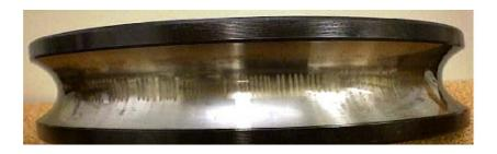
Figure 18 - 'Characteristic 'fluting' wear of inner race
