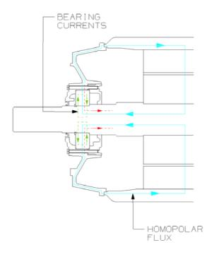
Figure 3 - Homopolar fluxes around stator, rotor and shaft
