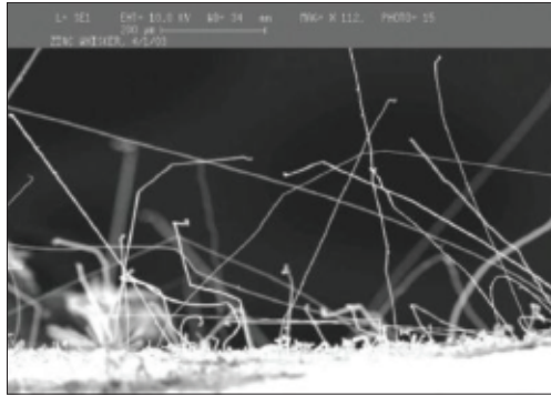
Figure 27 Microscopic image of zinc whiskers (image courtesy of the NASA Electronic Parts & Packaging Program)
